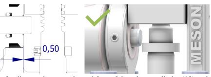
If there is too far distance between the end face of the release cylinder (13) and the bonnet (8) inner face, review must be done as to what is hindering the correct positioning of the release cylinder (13) and counted actions taken to avoid spontaneous activation of the release mechanism.
