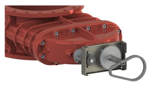
7. Tighten the screws connecting the hydraulic motor the bottom plate.
