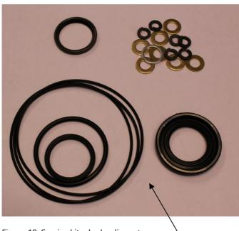
Figure 19. Service kit – hydraulic motor.
