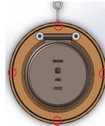
Figure 1, Where to push down the O-ring.
