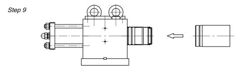
Mount the cylinder back on the actuator.
