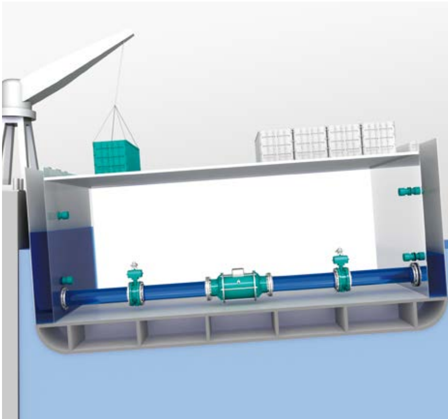
The anti-heeling system keeps the ship upright during cargo operations
